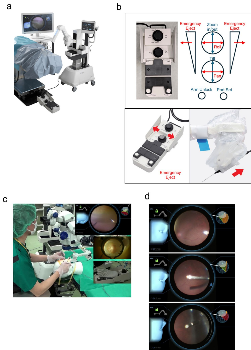
Fig. 1 Intraocular endoscope-holding robot OQrimo®. a The total system features of OQrimo® that stably hold an intraocular endoscope or illumination device. The surgeon can operate OQrimo® using a foot controller while viewing the endoscope screen. b Foot controller with pan, tilt, zoom in, zoom out, roll, arm unlock, port set, and emergency eject functions (upper panel). When the operator senses danger, they can kick either the left or right wall of the foot controller (lower left panel), allowing OQrimo® to perform an emergency retraction of the instrument inserted into the eye (lower right panel). The reaction time for this process is 0.035 seconds. c OQrimo® is designed for use in combination with a wide-viewing fundus observation system such as RESIGHT®. Upper left: View of the instruments at hand. Each tool can be inserted without interference. Upper
